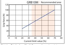
Total value of both fingers when grip point (Note) lotal value of both fingers when grip point distance (L, H) is 0. Guideline values. There is variation of 0 to 60%. In particular, current limit values set outside the recommended range (colored part of the graph) are more likely to lead to variation. For gripping (pushing), the speed is fixed at Smm/s. (Note)
