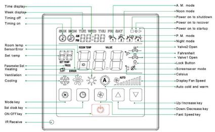
Setting parameter No. 13, the selection of the fan coil system has to be done. 2-pipe or 4-pipe systems can be selected.
