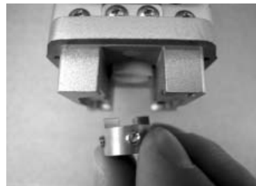
Inserting the coupling (with screws)
