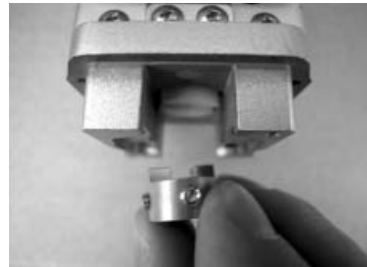
Inserting the coupling (with screws)
