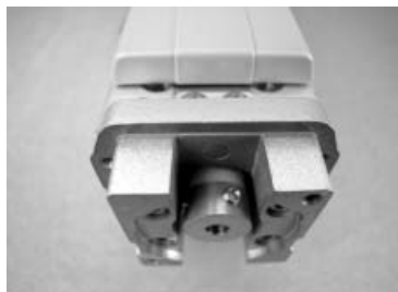
Inserted coupling (with screws)
