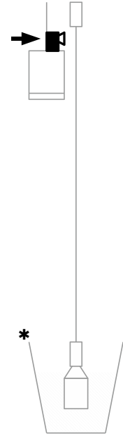
Figure 14: Step 2 Install APS sensor on cabin (side view)
