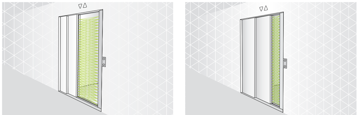
Dynamic application - criss-cross beams active up to complete door closure
