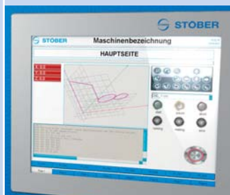
Parameterization directly on the machine (MC6 motion controller with touch screen panel)
