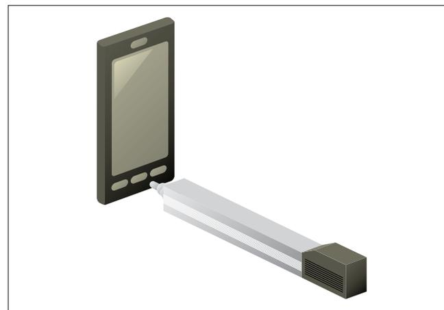
This ERC3-based system conducts life test on electronic equipment. The push speed and force can be changed according to the product.
