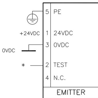
**\* If the TEST function is not required by the application, connect pin 2 of the emitter to +24Vdc.**
