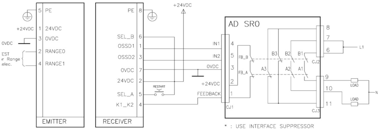
**Connection of VXL Emitter (modification of the above schematics)**
