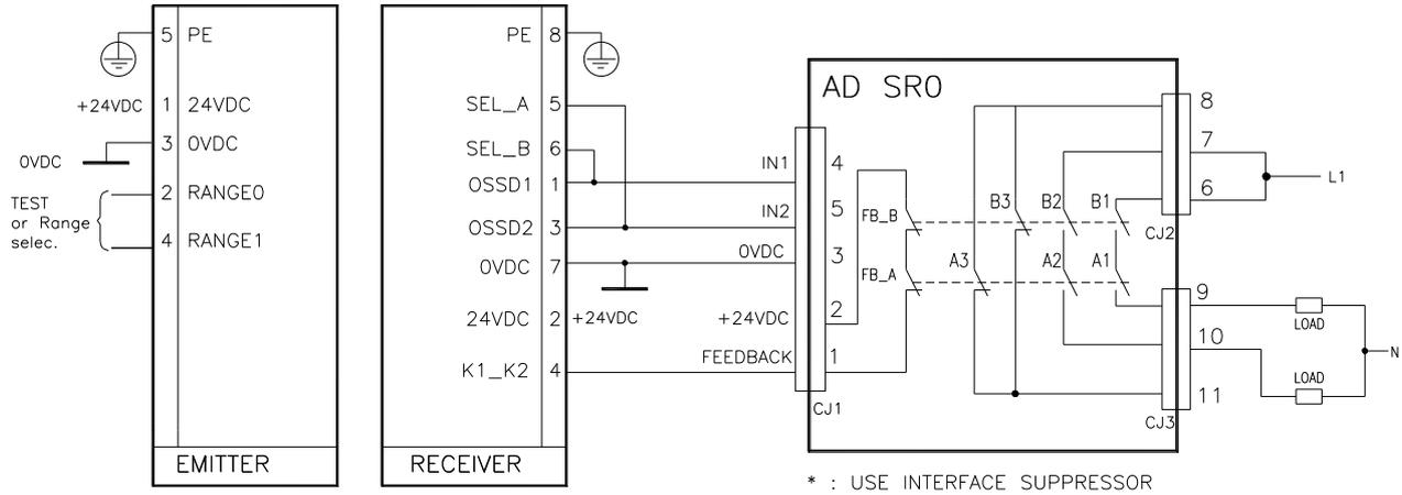
**Example of connection of the AD SR0 module with AX / VX / VXL safety light curtain in MANUAL operation mode**
