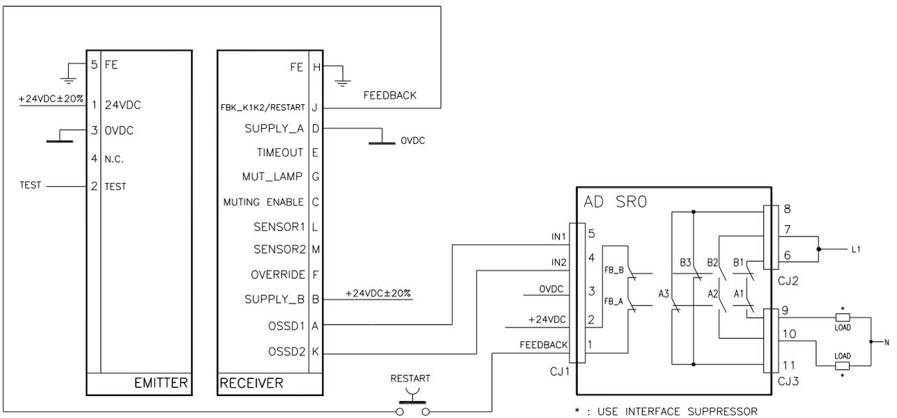
**Example of connection of the AD SR0 module with EOS4X safety light curtain in AUTOMATIC operation mode**
