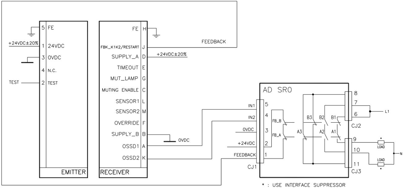
**Example of connection of the AD SR0 module with MXL safety light curtain in MANUAL operation mode**
