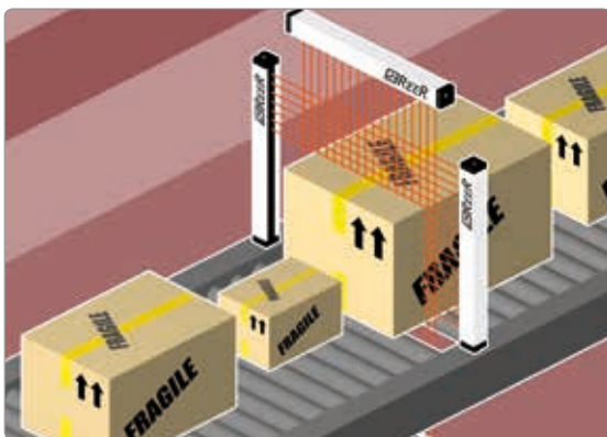
Two-dimensional detection of objects in transit on conveyor systems with use of 2 light curtains. If necessary, the calculation of the volume can be made by means of a third horizontal light curtain, or considering the transit speed
