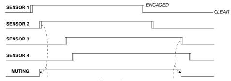
Figure 8 Sequential muting: activation sequence.
