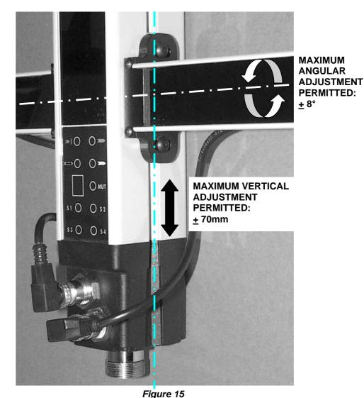
NOTE: For installations that do not require any particular adjustments, the ML and MT models are pre-aligned and do not require further regulation.
