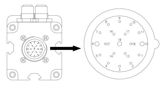
Make sure the M23 connector is screwed down tightly to ensure correct barrier operation! (4 turns)
