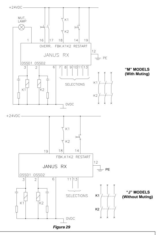
In order to assure a correct barrier operation, <u>it is necessary</u> to connect the pins 2 and 4 of the Emitter according to table 6 (page 20) and to the "TEST FUNCTION" paragraph of page 26. For correct operation (in the case of JANUS "M" without the use of Muting) the muting light must be connected (pin 1) and the Muting mode must be configured correctly (pin 7-8-9-10) following the indications in Table 13.
