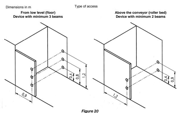
Protection of the opening with JANUS light curtain and mechanical side guards.
