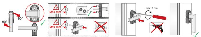
Put the window handle in the 90° position and rotate the cover by 90°.
