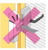
Because the handle can be turned only while it is pushed, the actuator is prevented from hitting the switch cover unit.
