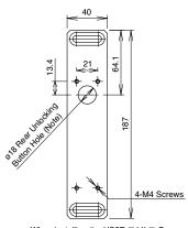
When installing the HS5E-□44L□-G (rear unlocking button type), provide a rear unlocking button hole on the HS9Z-SP51.
