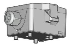
The leakage sensor lies with its own weight on the four contact feet. The detector electrodes are electrically insulated at the lower end, whereby a surface condensation is not detected. The height of the insulation can be variably adjusted, which makes it easy to adapt to local conditions. For height adjustment, please note that only the plastic adjustment screw (insulation) is moved in the direction of rotation and not the detector electrode (hexagonal spacer sleeve).
