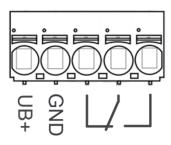
The representation of the relay contact indicates the operating state "Devices connected to voltage supply and no leakage is detected". The relay is energized in this operating state. When condensation or when switching off the operating voltage, it falls off.
