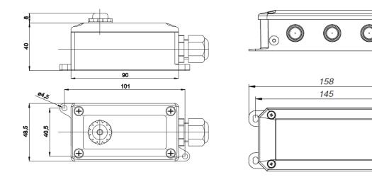
Housing IP65, Type: 200 Housing IP65, Type: 300
