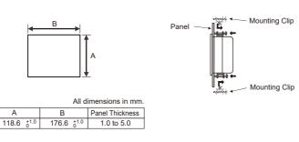
Place the HG2J-7U in a panel cut-out and fasten with the attached mounting clips at the four places to a specified torgue of 0,5 to 0,6N-m uniformly.
