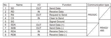
HG2J-7U is not equipped with terminating resistor. Insert a terminating resistor of an appropriate value (about 100 to 120 Ohm, 1/2W minimum) between terminal number 8 (RDA) and terminal number 9 (RDB), if necessary,
