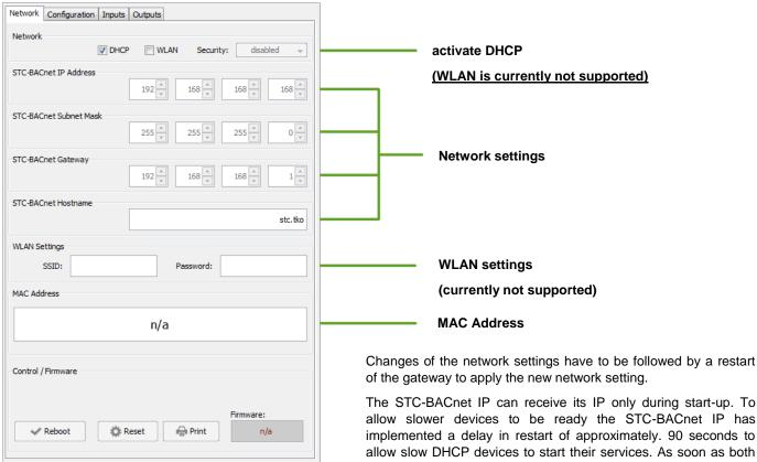
The STC-BACnet IP can receive its IP only during start-up. To allow slower devices to be ready the STC-BACnet IP has
