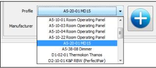
Select the tab "outputs" and select a SAB type telegram (A5-20-01 MD15) from the drop-down list and add it to the output list.
