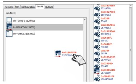
The teach-in of an valve actuator works in both directions. The SAB does need to learn the ID of the Message Server and the STC-BACnet IP needs to know the SAB'S ID. Therefore the SAB will show up in the inputs section as well as in the outputs. It's status telegram will show up in the inputs, the new position telegram will be sent from the outputs.
