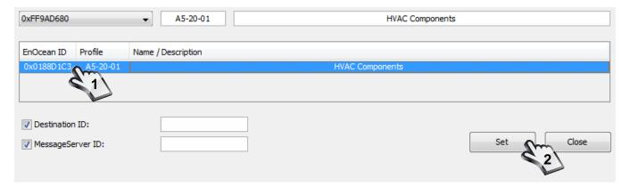
The Message Server does forward data to a particular SAB only, which is done by using addressed telegrams. The address must be set by selecting Destination and the ID of the SAB valve actuator.
