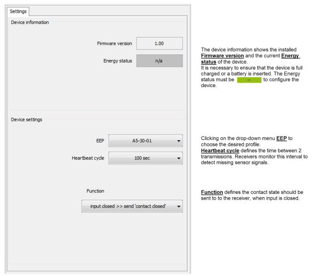
Right-click on the device icon and send configuration to initiate the transfer of the new settings. As the sensor will be sleeping it will need to be woken up by pressing the LRN button. Once the configuration has been transferred successfully into the device the sensor will be highlighted in green. Highlighted in Red indicates a problem during the transmission.
