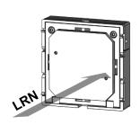
After delivery the room operating unit might be in default shipping mode, in this case press the learn button (<1 second) at the rear of the device [Signal telegramm will be send. SIG -> 0x0F // shipping mode deacticvated].
