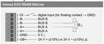
With alternating voltage, the correct polarity must be ensured!
