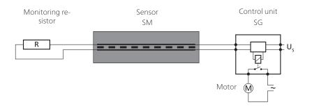
The monitoring resistor must be compatible with the control unit. Standard value is 1k2. 8k2 and 22k1 are also available.
