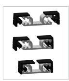
Tip 1: Brush the aluminium profile and clip bars or T-foot with a volatilizing **lubricant** (e.g. water with washing up liquid).
