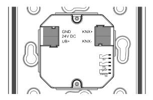
On the side of the lower part of the housing there is a socket connector for connecting up to 3 digital inputs (optional as an NTC10k). The connection is made via a pre-assembled female connector (included in delivery).
