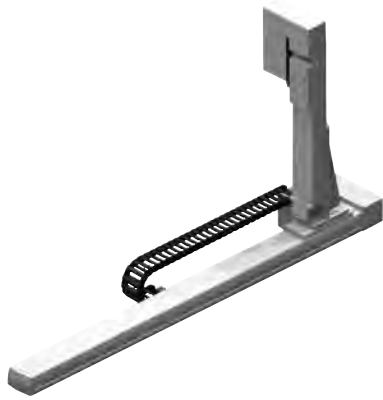
Wiring 1 with cable track
