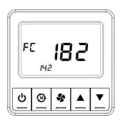
During device start-up the version and type number are displayed on the start screen for a short time.
