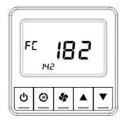
During device start-up the version and type number are displayed on the start screen for a short time.
