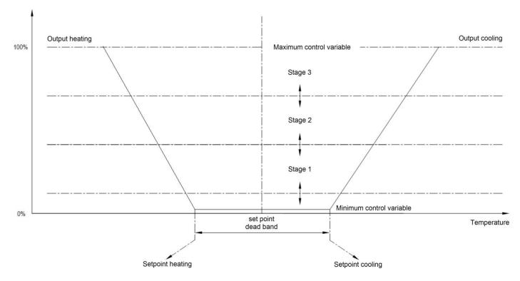
Minimum and maximum control variable are set in the parameter table (item 8 & 9). PI loop's output will be converted to an analogue voltage depending on valve type:
