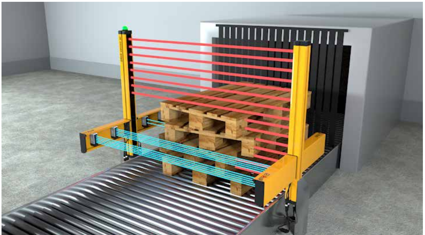
Palletizer with irregular pallets transit showing a Safegate with MZ Muting brackets (M 5 multi-beam photocells)
