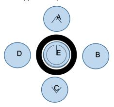
Menu navigation on the touch-surface is performed by pressing the buttons "up" (A), "down" (C), "left" (D), "right" (B) or the power button. Choose the desired parameter and press "right" (B) to open up the submenu. The menu will default after 30 seconds if no button is pressed. To exit the menu select the header line and press "left" (D)
