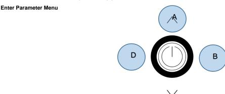
The configuration menu is activated by simultaneously pressing the buttons "up" (A), "left" (B) and "right" (D) for at least 3 seconds.
