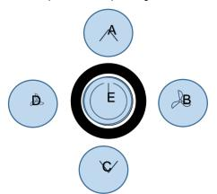
The buttons (A) and (C) change the setpoint in the range ± 3 ° C (default setting, configurable).
