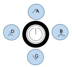
The configuration menu is activated by simultaneously pressing the buttons "up" (A), "left" (D) and "right" (B) for at least 3 seconds.
