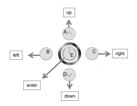
Menu navigation on the touch-surface is performed by pressing the buttons "up" (A), "down" (C), "left" (D), "right" (B) or the power button. Choose the desired parameter and press "right" (B) to open up the submenu. The menu will default after 30 seconds if no button is pressed. To exit the menu select the header line and press "left" (D)
