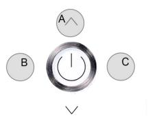
The configuration menu is activated by simultaneously pressing the buttons "up" (A), "left" (B) and "right" (C) for at least 3 seconds.
