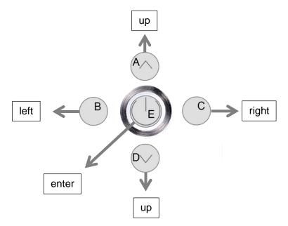
Menu navigation on the touch-surface is performed by pressing the buttons "up" (A), "down" (D), "left" (B), "right" (C) or the power button. Choose the desired parameter and press "right" (C) to open up the submenu. The menu will default after 30 seconds if no button is pressed. To exit the menu select the header line and press "left" (B)
