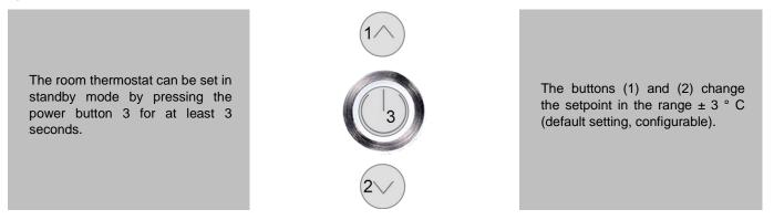
With power-button (3), the device can be set in standby mode by pressing the button (if keycard-switch is NOT used). If the button is used as a occupancy button, the button must be pressed for at least 3s, in all other cases, a short actuation is sufficient. In standby mode, the display and all outputs are switched off (controller deactivated). The frost and heat protection monitoring remains active.
