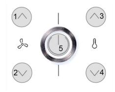
The buttons (3) and (4) change the setpoint in the range  $\pm$  3  $^{\circ}$  C (default setting, configurable).
