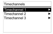
Menu navigation through the menu is performed by pressing the buttons on the touch-surface "up" (A), "down" (C), "left" (D), "right" (B) the power button. The menu will default after 30 seconds if no button is pressed. To exit the menu select the header line and press "left" (D)
