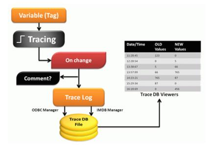
Data relating to each status change occurred for each single variable Tag is files in the appropriated files (one Table for each Tag) and is made available to the user through display window objects which can be inserted on screen.
