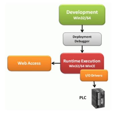
The development environment (Design Mode) produces projects based on open architecture (XML). The project interpreter is called Runtime which executes the projects created in the development environment.
