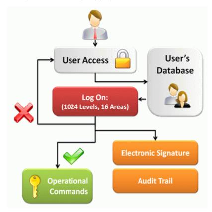
Access security is managed by enabling the password management using the Users and User Groups Resource general properties. Therefore, any command object can require user authentication (Log On) when defined with a hierarchy protection level in its Access Level properties. The will protect command activation by subjecting them to verify Log On access privileges of user trying to activate command before allowing them to do so.
