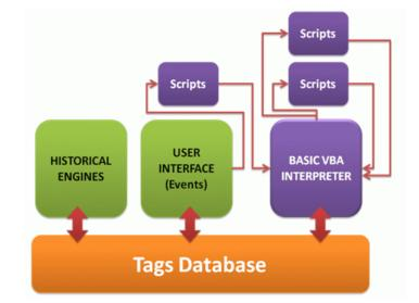
Movicon comes integrated with a software component called WinWrap Basic which allows you to interact internally with routine applications in Basic language. In addition to the script functions provided by this component there are also all those belonging to Movicon which are needed for managing project resources and objects.
