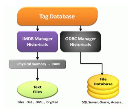
Data recording on file can be managed according to these two different write on file modalities which can be set as pleased:
