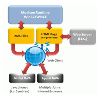
Movicon Web Client© is based on the Java Thin Client architecture and exploits the web Services communication for visualizing and/or controlling your automation system from any client station in LAN or WAN.
