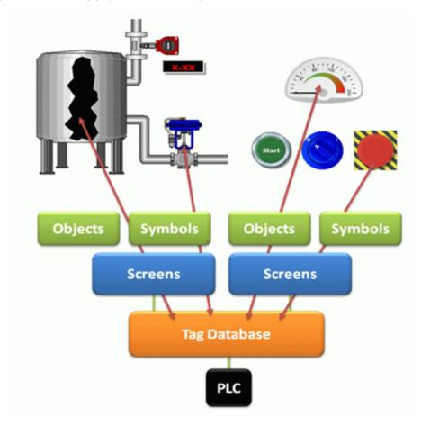
The screen windows are operator interfaces and can be activated for operator use in "Maximized Screen" and "pop-up" mode being windows that display on top of other windows. Movicon also has an interesting object called the "Embedded Screen' through which screens can be displayed within other screens.
