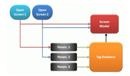
The parameter files are simple text files (UNICODE format) within which the associations between "Alias Parameters" and "Effective-Variables (Tags)" are specified. These files are created by the programmer directly in Movicon, or externally.
