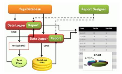
Movicon has integrated the "Report Designer" totally free to allow users create autonomously reports relating to the Movicon databases. In addition, Movicon still remains compatible with the "Crystal Report™" report engines which, however, is not integrated in Movicon and must be purchased separately for creating the reports desired. Textual Reports are also compatible with the WinCE environment where they can be created with great ease and simplicity.
