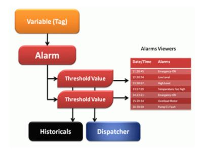
The Movicon Alarm management is completely configurable to adapt to any application requirement. The alarm property default configuration conforms to the ISA-S-18 specifications. The project alarms are objects which can be set with diverse thresholds. Alarm activation can be evoked by a fixed threshold value or by another variable.
