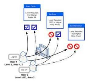
Project users must be inserted in groups. Some properties are made available both for User Group levels and single user levels. This eases propagating the same properties to the all users of the same group to then also differentiate these properties for each group user member or single user later on.
