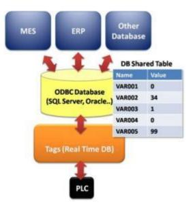
Movicon will create a table in the selected database format, in which a record will be reserved for each variable enabled with ODBC sharing. Each table column will report the current value or the statistical value of the corresponding variable.
