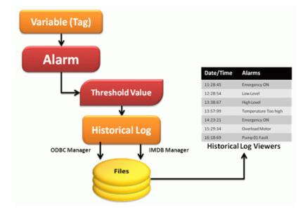
The Acknowledge (Ack) or reset operations in each alarm can be configured, just as their styles and functioning modalities can be completely configured.
