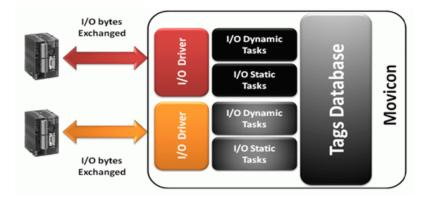
The communication drivers manage connections between the device areas and the Movicon variables using links normally defined in the Tag's properties (Dynamic Task), but communication tasks (Static Task) can also be defined to permit associations between device memory data "groups" and Tag groups.
