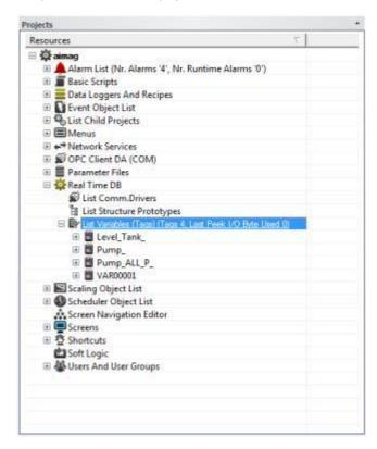
Each resource can be accessed and configured in Project edit mode through the **Project Explorer** window (as seen above). Each resource, according to function type, can be configured through its **Properties Window** and can contain specific elements and objects which are also configurable through their relating properties.
