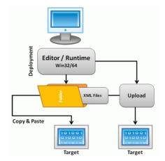
The Movicon platform architecture is built with a software structure capable of generating XML format based project files, using a simple and intuitive approach involving object-oriented programming.
