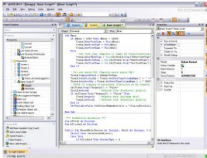
*Movicon integrates the VBA language with support to multithreading, safe mode and parameterization. Many other tools included such as the debug and thread priority functions.*
