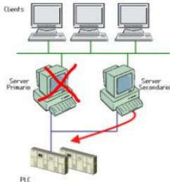
*A simple redundancy architecture*
