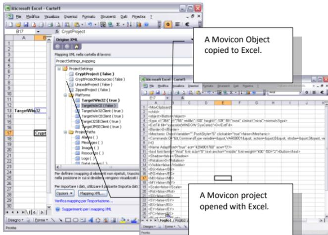
Each object's XML structure can be accessed directly through the XML Explorer window with the Movicon editor to modify its properties textually.
