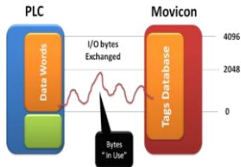
*This chart shows a project connecting 4096 I/O bytes simultaneously, but only 2048 of them actually go into use and not more. Therefore a license with 2048 I/O bytes is needed.*
