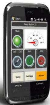
phone normal networks (GSM/GPRS, UMTS). In addition to displaying screens on the phone, the Web Client Midlet also provides the main services for accessing information on the server in a much more simpler way compared to a normal Web Client.
