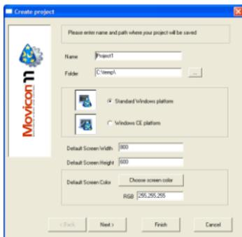
Each project setting automatically created by the Wizard can be modified afterwards though the relating properties of each single resource.
