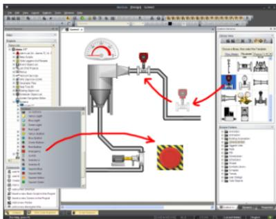
*The object-oriented programming allows you to use the drag&drop techniques for inserting symbols and objects and assigning Tags. The configuration procedures are done through the properties window.*
