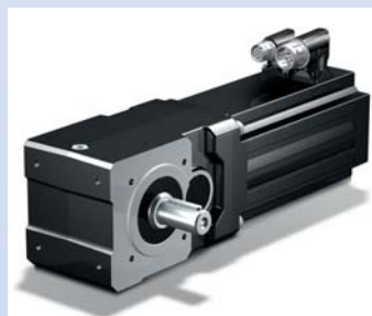
SMS KL helical bevel geared motor Acceleration torque: 15 – 65 Nm Backlash < 16 – 25 arcmin Super compact and of wide ranging application
