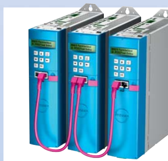
POSIDYN® SDS 5000 servo inverter In multiple axis operation (electronic shaft) with Integrated Motionbus and IGB network. The network (up to 32 axes) is set up automatically on switch on You will find information on motion control interfaces for higher level controllers in the internet: www.stoeber.de > Products > Software/Download > Fieldbus
