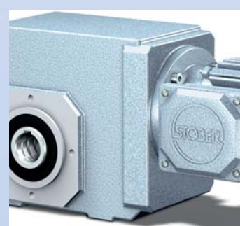
MGS K helical bevel geared motor Specific surface treatment for hygiene applications. Output designed as hollow bore or solid shaft in stainless steel 1.40.57. Enclosure type IP 56 Special FoodTech version
