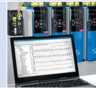
Central commissioning of a CODESYS multi-axis application
