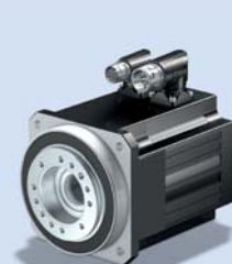
SMS PY Planetary Geared Motor with Hollow Shaft Acceleration torque: 47 – 500 Nm Backlash: ≤ 3 – 4 arcmin Super compact, maximum power density
