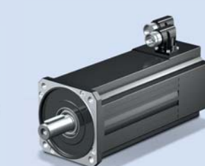
ED Synchronous Servo Motor Slim design, high torque 6 sizes: ED 202 – ED 808 Stall torque: 0.48 – 86.4 Nm Optimized for applications with high dynamics
