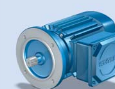
MGS IE2 Asynchronous Motor 14 selection parameters (standard) Motor power: 0.75 – 45 kW Optional: brake, forced cooling fan, incremental encoder or multturn absolute encoder
