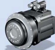
SMS PH(A) Planetary Geared Motor Acceleration torque PH(A): 41 – 2 000 Nm Backlash PH: ≤ 3 – 4 arcmin Backlash PHA: ≤ 1 – 2 arcmin Designed for high-performance servo drives
