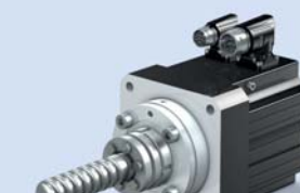
EZS Synchronous Servo Motor Rotating threaded screw drive Motor shaft as blind hole hollow shaft Feed force at standstill: 923 – 26 138 N Designed for high thrust forces
