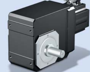
SMS K Helical Bevel Geared Motor Acceleration torque: 33 – 6 875 Nm Backlash: reduced class I ≤ 1.5 – 6 arcmin Versatile with flanged, solid or hollow shaft
