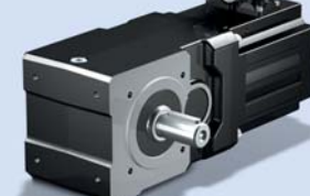
SMS KL Helical Bevel Geared Motor Acceleration torque: 33 – 60 Nm Backlash: ≤ 16 – 20 arcmin Super compact drive solution for small servo drives
