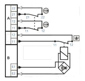
**2NC Model**For monitoring the guard locking (built-in solenoid) slow-action switching contact 2 NC
