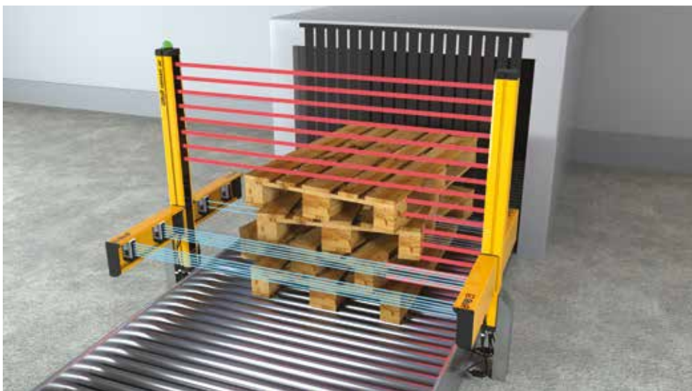
Palletizer with irregular pallets transit showing a Safegate with MZ Muting brackets (M 5 multi-beam photocells)
