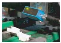
Application laser sensor "Midi" Permanent monitoring of plastic pieces on attendance in a transportation system. As part of a fully automatic assembly line the sensor identifies housing feed previous to the final assembly.
