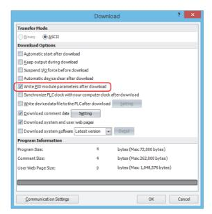
Click the check box on the left of **Write PID module parameters after download** and click **OK** button. The user program will be downloaded. After downloading the user program, the PID module parameters will be automatically written to the data registers in the CPU module and the PID module connected to the CPU module.
