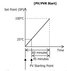
When program control is started, the control starts from the PV starting point (25°C of the process variable).
