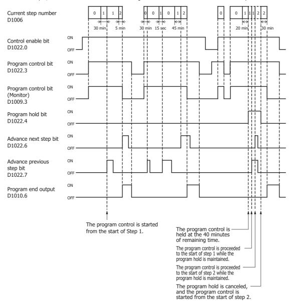
**Note:** The PID module executes all steps 0 to 9 even if the step times of steps are zero. When the program control is terminated, nine is stored in the current step number of Block 0.
