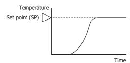
In reality, the ideal temperature control shown in Figure 1 on the previous page is almost impossible to achieve due to a number of complicated factors such as thermal capacity, static characteristics, dynamic characteristics and disturbances.
