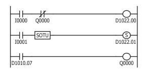
While external input I0 is on, CH0 control is enabled. When Q0 (CH0 control upper/lower limits alarm output) is on, CH0 control is disabled.
