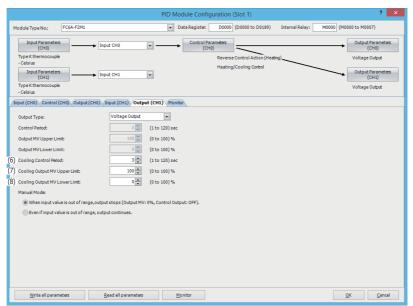
Output parameters of CH0 control are described here. When the heating/cooling control is enabled, the control period and the output manipulated variable (MV) upper and lower limits of CH1 are disabled. The parameters (5) to (7) are enabled.
