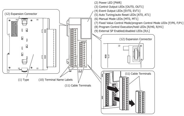
The content in brackets is the LED indicator name on the PID module.
