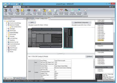
Select the expansion module or cartridge to insert in the expansion modules and cartridges list and drag and drop it to the module configuration area.
