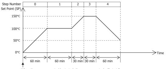
When the program control is started, the program control will start from 0°C of the set point (SP) configured with "Set Point (SP) when Program Control Starts" regardless of the current process variable (PV).
