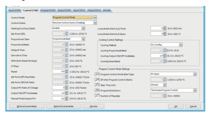
Control parameters of CH0 control are described here. When the program control mode is selected as the control mode, parameters for the fixed value control mode, such as the set point (SP), proportional band/proportional gain, or integral time, are disabled. The parameters for the program control mode (23) to (27) are enabled.
