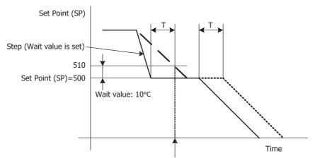
Moves to the next step when process variable (PV) reaches 510°C
