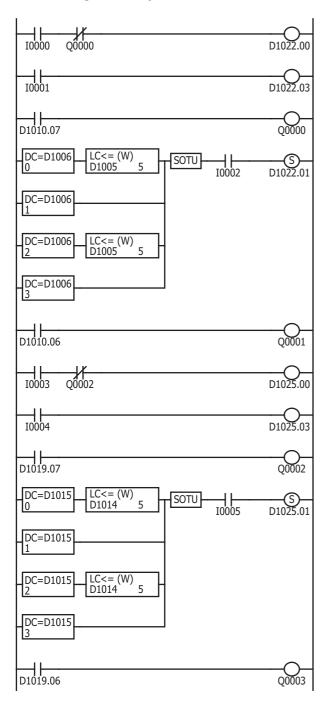
While external input I0 is on, CH0 control is enabled. When Q0 (CH0 control upper limit alarm output) is on, CH0 control is disabled.
