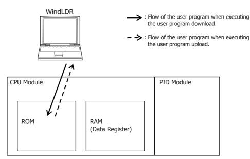
\*1 When the **Write PID module parameters after download** check box is selected in the **Download** dialog box, the parameters will be written after the user program is downloaded to the CPU module.
