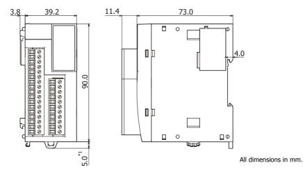
\*1 9.3 mm when the hook is pulled out.
