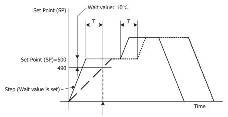
Moves to the next step when process variable (PV) reaches 490°C
