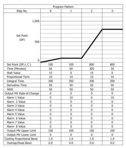
When the program pattern is configured as shown in the above table, the following control is performed at each step:
