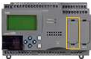
FT1A-ModBUS RTU (Master)
