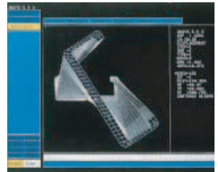
Deformation of competitor's base structure under the same amount of force.
