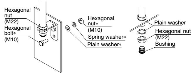
The parts marked with \* are not supplied and should be prepared by the user.
