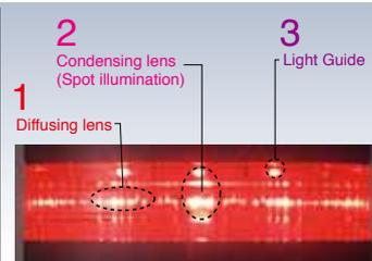
By combining a diffusing lens, which diffuses the light broadly, with a condensing lens, a super bright area is created enabling high visibility. Also, the illumination through the light guide enhances the visibility when the Signalight is viewed from below.
