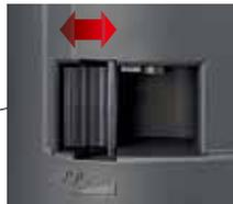
Sound volume adjustment (adjustable within a range of 70 to 90 dB)
