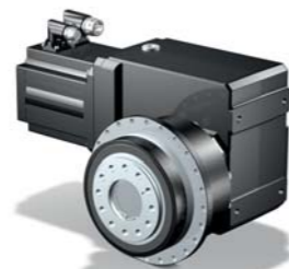
SMS PHQK Right-Angle Planetary Geared Motor Acceleration torque: 230 – 10,000 Nm Backlash : < 3.5 – 4 arcmin Quattro Power in the compact right-angle design
