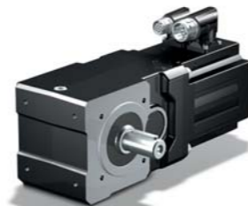
SMS KL Helical Bevel Geared Motor Acceleration torque: 15 – 65 Nm Backlash : < 16 – 25 arcmin Super compact drive solution for small servo drives
