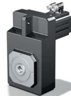
SMS F Shaft-Mounted Helical Geared Motor Acceleration torque: 23 – 1,100 Nm Backlash: reduced < 5 – 8 arcmin Servo axis with parallel axle offset
