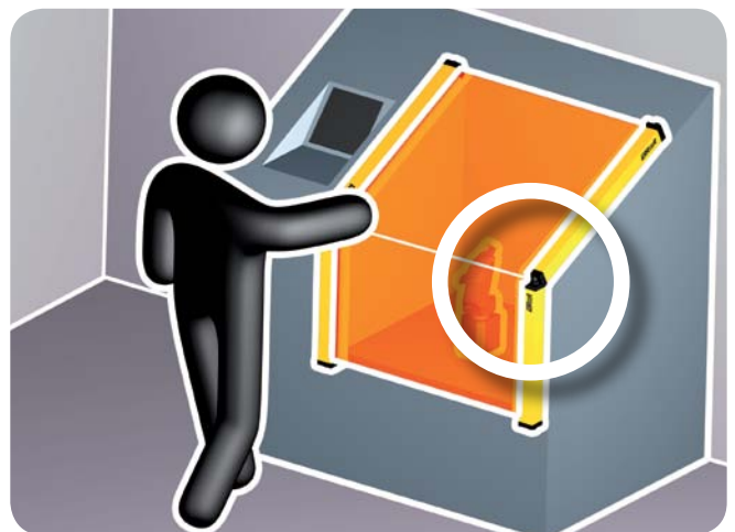
The resolution is maintained (up to 40 mm) in the junction between the 2 protected areas
